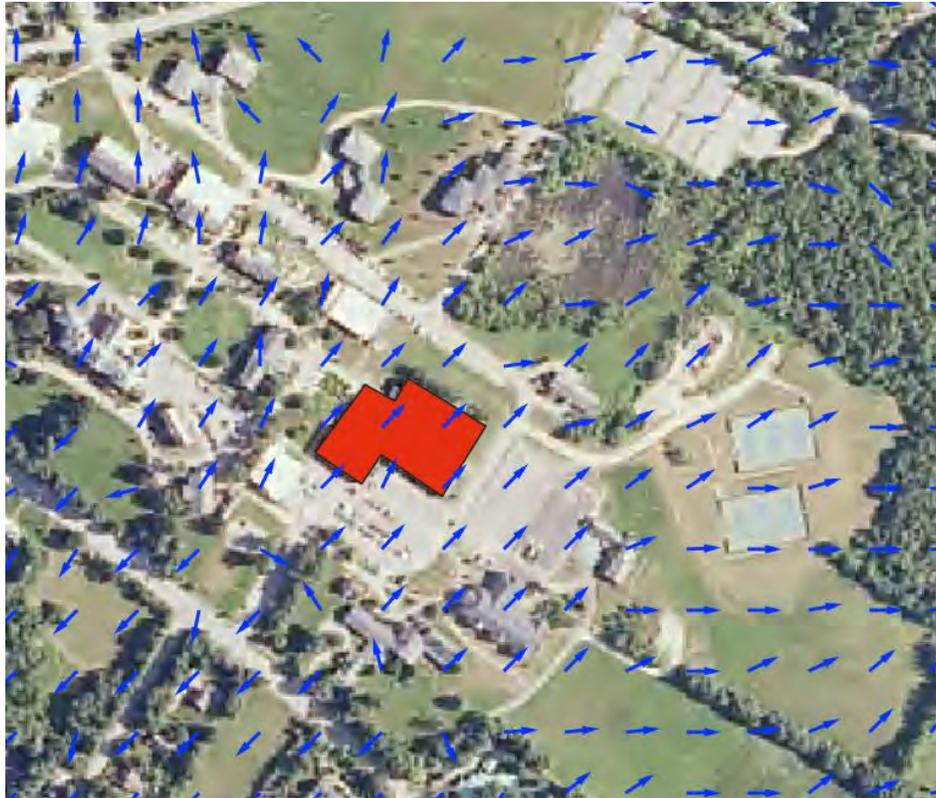
Figure 26. The flow of runoff based on the location of the Hogan Sports Center. The blue arrows represent the direction of runoff flow.
